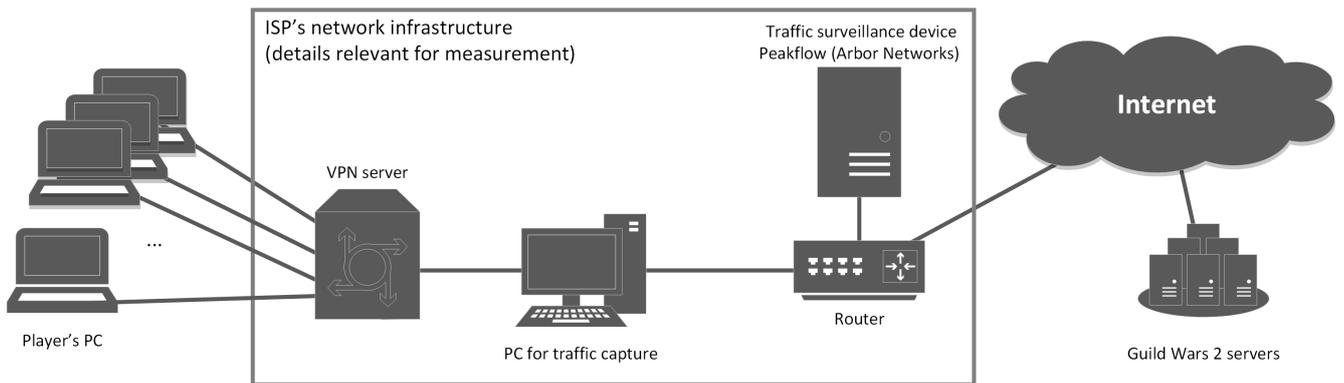
Fig. 1. Measurement setup
