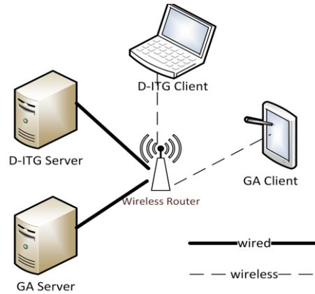
Fig. 3 Laboratory testbed
