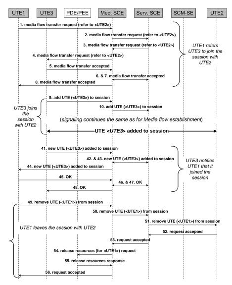
Fig. 4 The Change of user terminal signaling procedure
