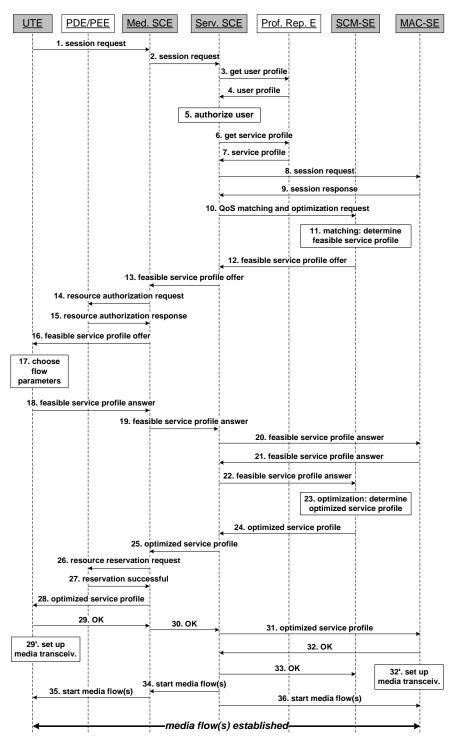
Fig. 3 The Media flow establishment signaling procedure
