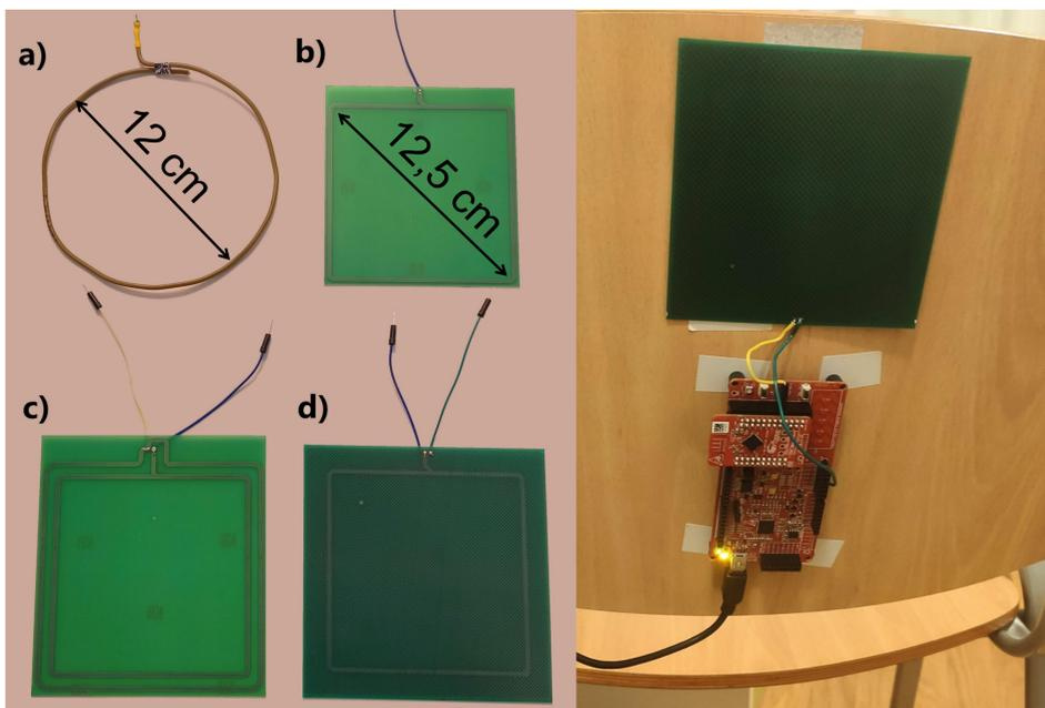
Ground loop reduces noise and improves ESD resistance, while hatched shield surface reduces parasitic capacitance and isolates signal loop from foreign objects. The microcontroller performs filtration of the signal using 1st order IIR filter and the ALP filter. All sensor surfaces can detect movement at 20 cm distance.
