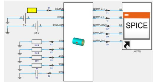
Within the **CST Studio Suite**, the upper arm was modelled as a concentric cylinder, along with the line action potential source. The preprocessing circuit is connected with the geometry via Schematic interface.
