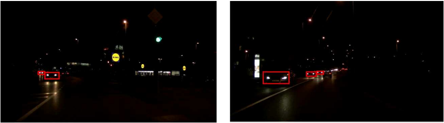
On-road night-time vehicle headlight detection and tracking.
