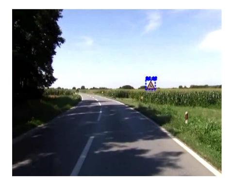
proof-of-concept for traffic sign detection based on Viola & Jones detector can provide reliable true detection rates and false positives rates in real time
