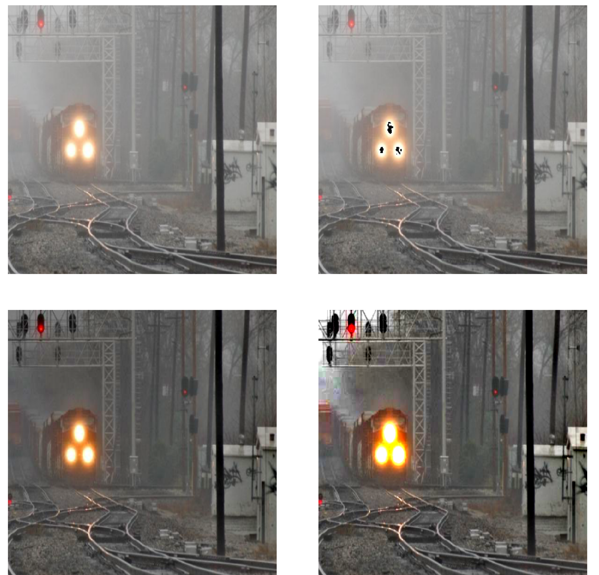
Figure: Top line shows the original hazy image (left) and the pixels included in estimation of airlight parameter A (right). The bottom image shows the dehazed images using the estimated, incorrect, A on the left, and a better value set by hand on the right.
