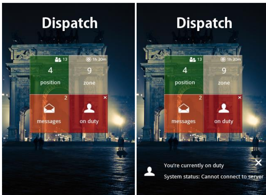
Figure 4.1.2.2: Taxi client user interface when coordinates are not being successfully communicated to the server. On the left is the default view (notice the “x” in the top-right corner of the status button). On the right is the view if the user clicks on the status button. The message displayed is different, depending on the error.
