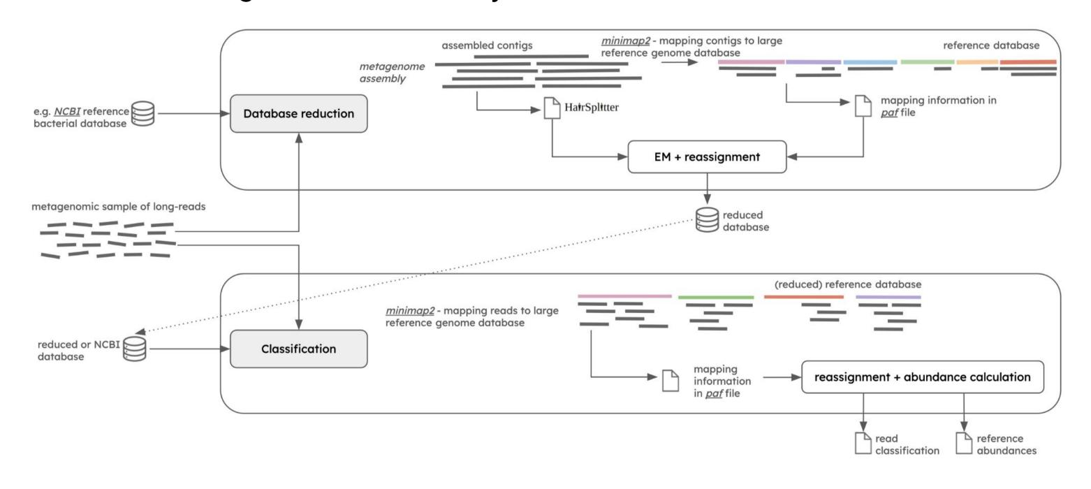
1) database reduction step - uses long-read assemblies and an EM-based contig-to-reference mapping strategy to identify relevant strains and build a reduced reference set
