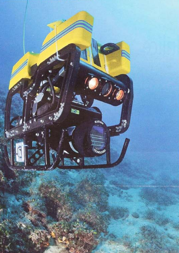
Robot Seamor Marine roni do 300 metara
