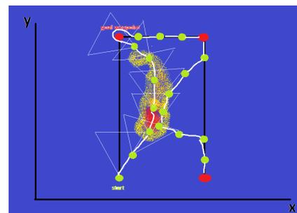
Fig. 1. An example of the AUV behavior in the presence of the interesting parts of the sea floor out of the lawnmower lines. Red circles denote the lawnmower's waypoints, green circles denote the vehicles position in discrete time intervals, while white lined triangles denote the forward-looking sonar range. Blue, yellow and red areas denote low, medium, and high information gain areas of the sea floor, respectively.
