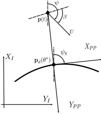
Fig. 2. Geometrical representation of the general path following problem [2].
