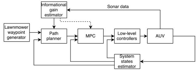
Fig. 4. Block diagram of the second proposed approach: Global path planner for computing the terminal cost in the MPC framework. Possible augmentation of the local MPC planner with the roughness values on the prediction horizon (dashed line).
