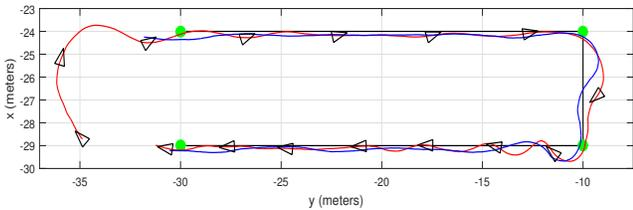
Fig. 6. Surface experiments. Reference lawnmower lines at a constant depth (black), defined by given waypoints (green markers). Vehicle's path while following the lines of the set lawnmower pattern: MPC controller (red), PID controller (blue). Heading of the vehicle controlled by MPC (black triangles).
