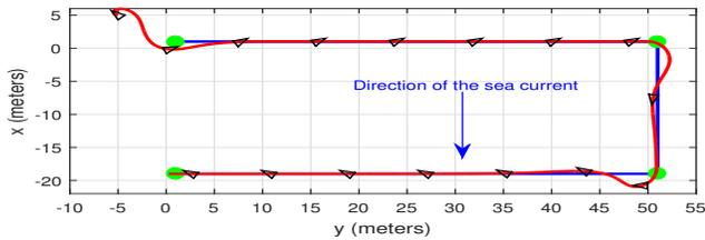
Fig. 5. Simulation results. Reference lawnmower lines at a constant depth (blue), defined by given waypoints (green markers). Vehicle's path while following the lines of the set lawnmower pattern (red). Vehicle's heading (black triangles).
