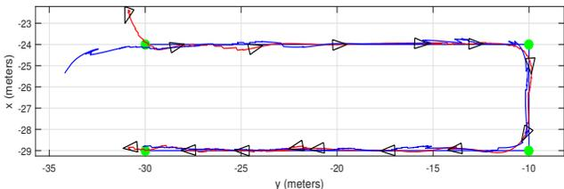
Fig. 7. Underwater experiments. Reference lawnmower lines at a constant depth (black), defined by given waypoints (green markers). Vehicle's path while following the lines of the set lawnmower pattern: MPC controller (red), PID controller (blue). Heading of the vehicle controlled by MPC (black triangles).
