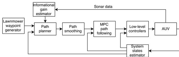
Fig. 3. Block diagram of the first proposed approach: Global path planner for computing the discrete path in the grid based map, which is then smoothed, and tracked with MPC path following control algorithm as a local planner.
