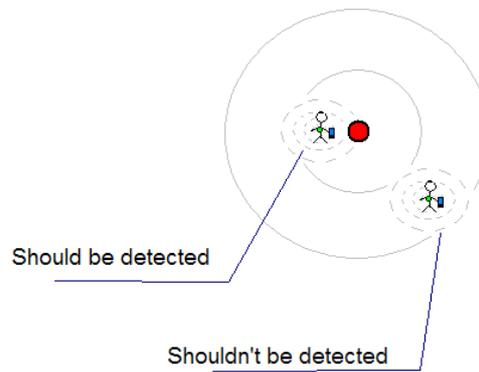
**Picture 2:** Dynamic mote radio range and detection
