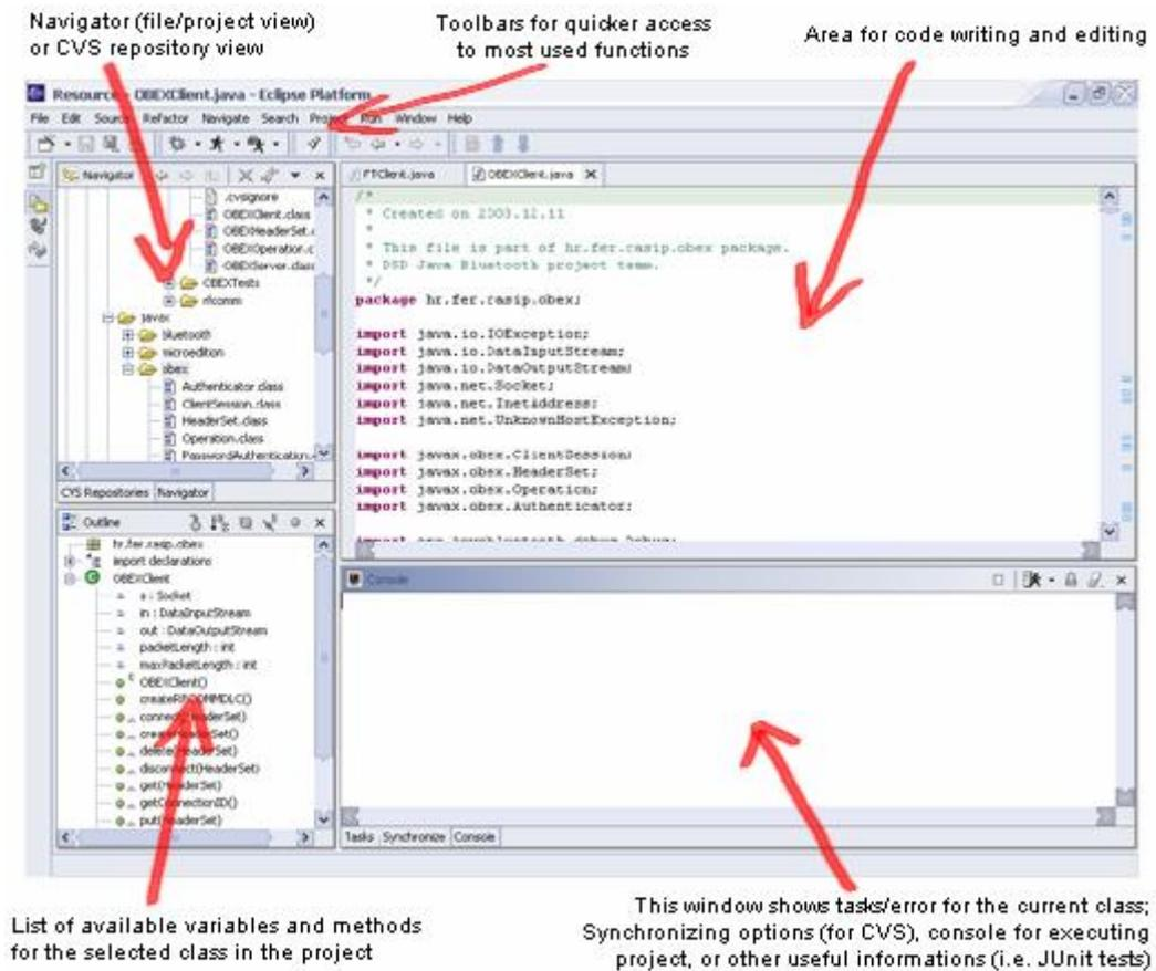
Fig. 6.1.1: Eclipse platform main window - Resource perspective
