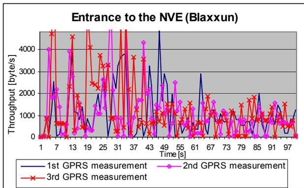
Figure 7. Throughput for “Entrance to the NVE” (download) action (3 GPRS measurement)
