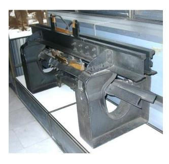
The collector was named "Budapest system" but its reliability was not too high because dirt could fall into the small ditch. Later this system was applied in Vienna and in Berlin, too.
