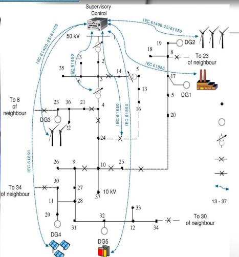
Communication model provided by *IEC* 61850 & *IEC* 61400-25 to describe the physical devices in the network model.
