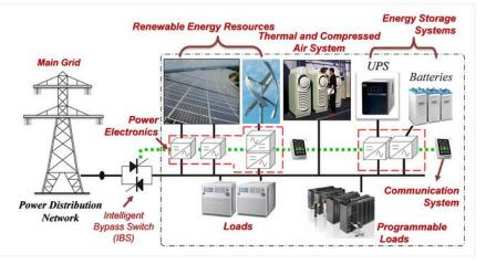
The MicroGrid research programme areas include AC and DC MicroGrids control and management, centralized and distributed control architectures, power quality and protections, multi agent systems, standard-based information and communication technologies, online optimization techniques and energy management systems. All of the foregoing can be also conceived within a problem based learning (PBL) education for Master, PhD students, and Industrial partners.
