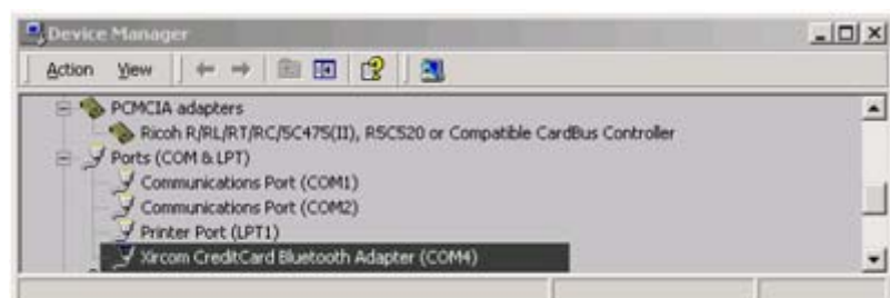
Fig. 8.1: Xircom CBT PC-Card installed as a virtual COM port
