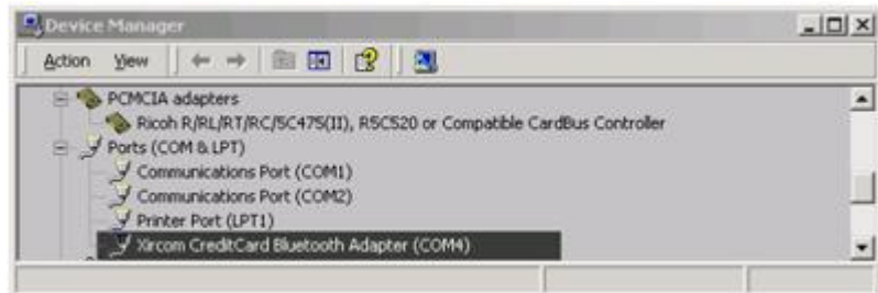
Fig. 6.1: Xircom CBT PC-Card installed as a virtual COM port
