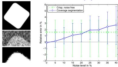
**Left:** (top) Synthetic test objects. (middle) Part of object with 30% noise added. (bottom) Coverage segmentation result for 30% noise. **Right:** Estimation errors for increasing levels of noise. Green is noise free crisp reference. Lines show averages for 50 observations and bars indicate max and min errors.
